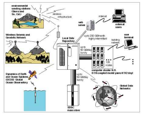
This is a schematic outline of the ITR Project ROADNet (Real-time Observatories, Applications, and Data management Network). ROADNet will enhance our capacity to monitor and respond to changes in our environment by developing both the wireless networks and the integrated, seamless, and transparent information management system that will deliver seismic, oceanographic, hydrological, ecological, and physical data to a variety of end users in real-time.
